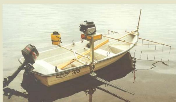
The **Dorocutter Wasse** is our smallest engine powered reedcutter. **Wasse** is the suitable reedcutter when small areas and different watersystems are maintained. The cutting deep, the drift of the knife, start and stop of the engine etc. are done from the drivers seat. The light construction makes transport and mounting easy. Rockreleaser is standard. The reed-rake is delivered as an accessory.
