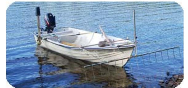
The **Dorocutters** can be used effectively with the **Reed rake**. The reed that sometimes disturb the propeller is steered away with the rake. The rake is used together with Hymo, Klippo, Wasse och Elis.
